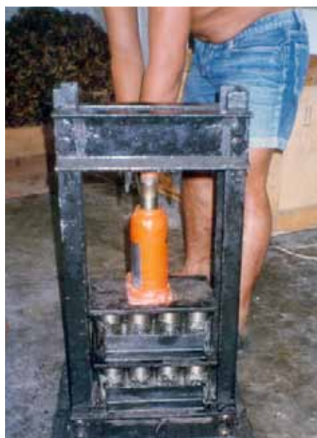
Figure 105. Briquetting machine (left) and manual briquetting press (right)
